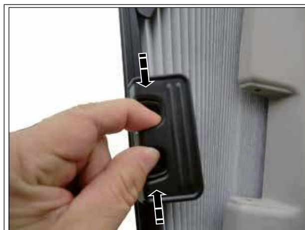
Fig. 19 Blackout blind, front and side windows
