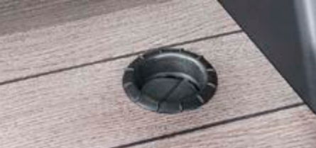
1 Additional warm air vents
