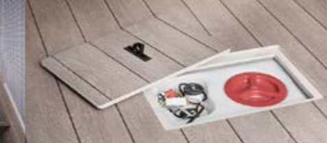
5 Fresh water tank cleaning hatch
