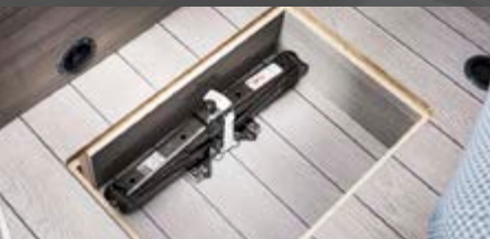
19 Jack in recessed compartment below the table
