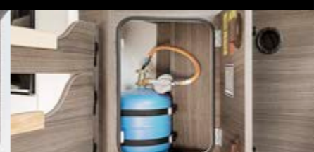
13 Compartment for 3 kg gas cylinders
